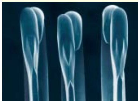
DUE TO WEAR OF THE LATCH GUIDANCE, INCREASED LATERAL LATCH PLAY
