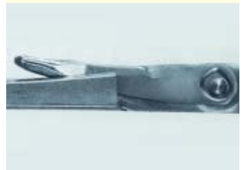
WORN LATCH HOLE, LATCH SHANK AND RIVET
